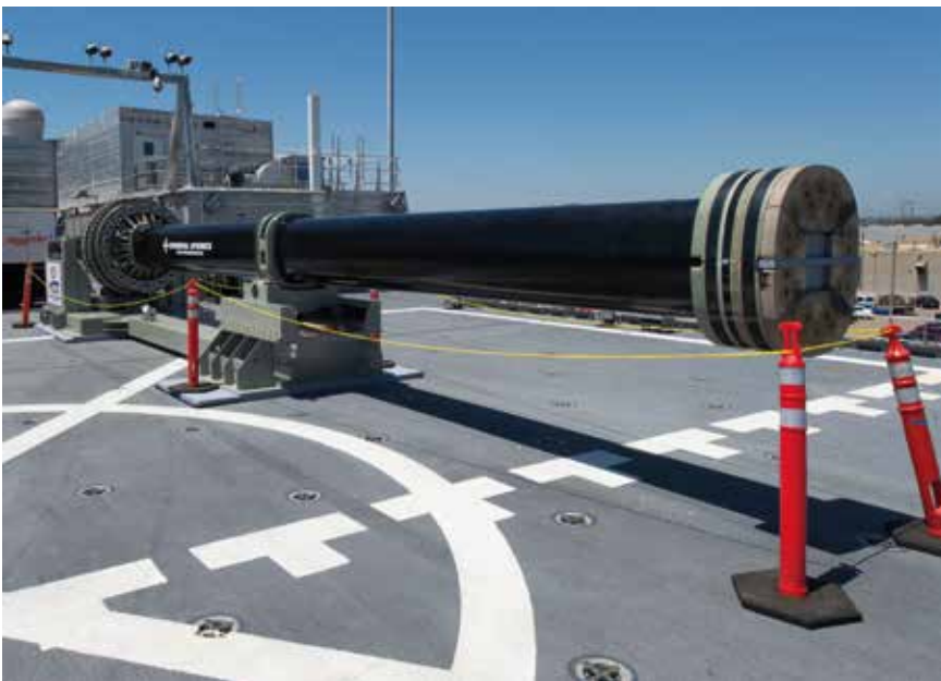
One of two electromagnetic railgun prototypes on display aboard Joint High-Speed Vessel USS MILLINOCKET (JHSV 3) in port at Naval Base San Diego on 8 July 2014
