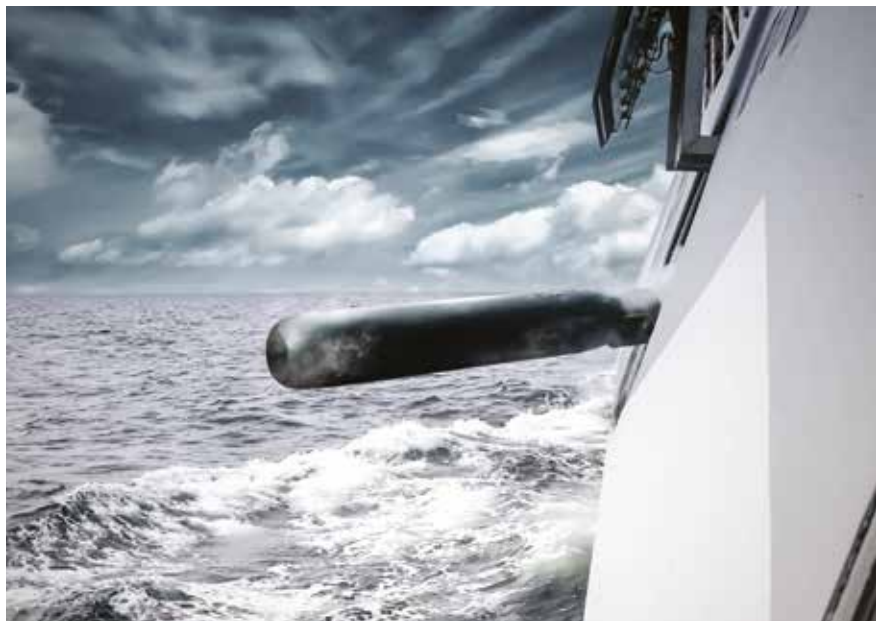
The new Saab Tp47 LWT was designed from the ground up with a modular design to integrate new technologies throughout its lifetime.
