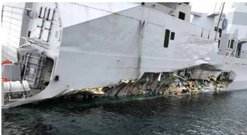
The giant gash in the frigate's starboard side. These images indicate that the frigate is seriously damaged and will require major repairs, if not being beyond repairs.
