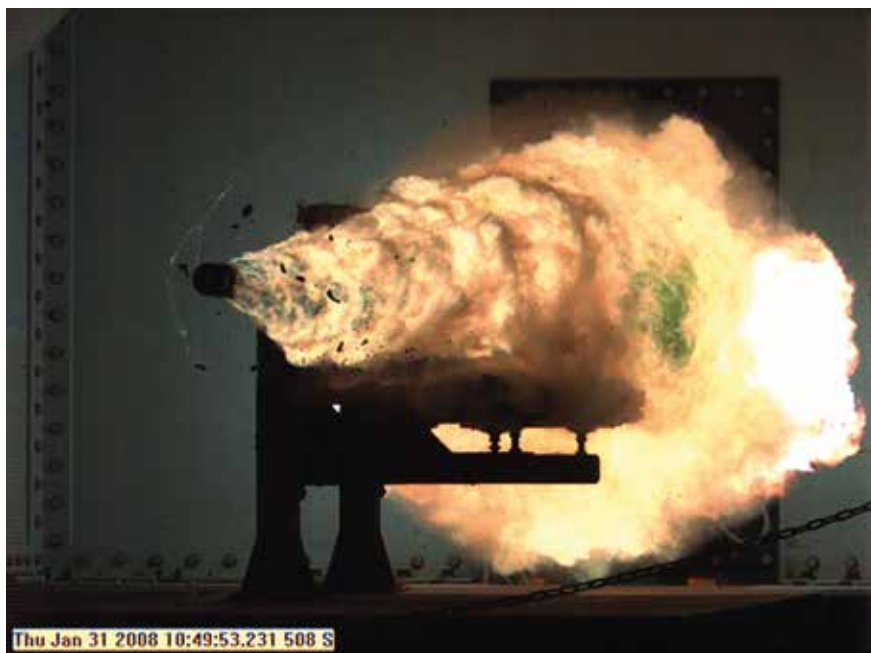
Photograph taken from a high-speed video camera during the record-setting firing of an electromagnetic railgun (EMRG) at Naval Surface Warfare Center, Dahlgren, Va., on 31 January 2008, firing at 10.64 MJ (megajoules) with a muzzle velocity of 2,520 metres per second
