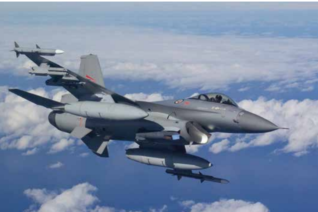
A Norwegian F-16A modified with SNIPER pod and IRIS-T missiles
