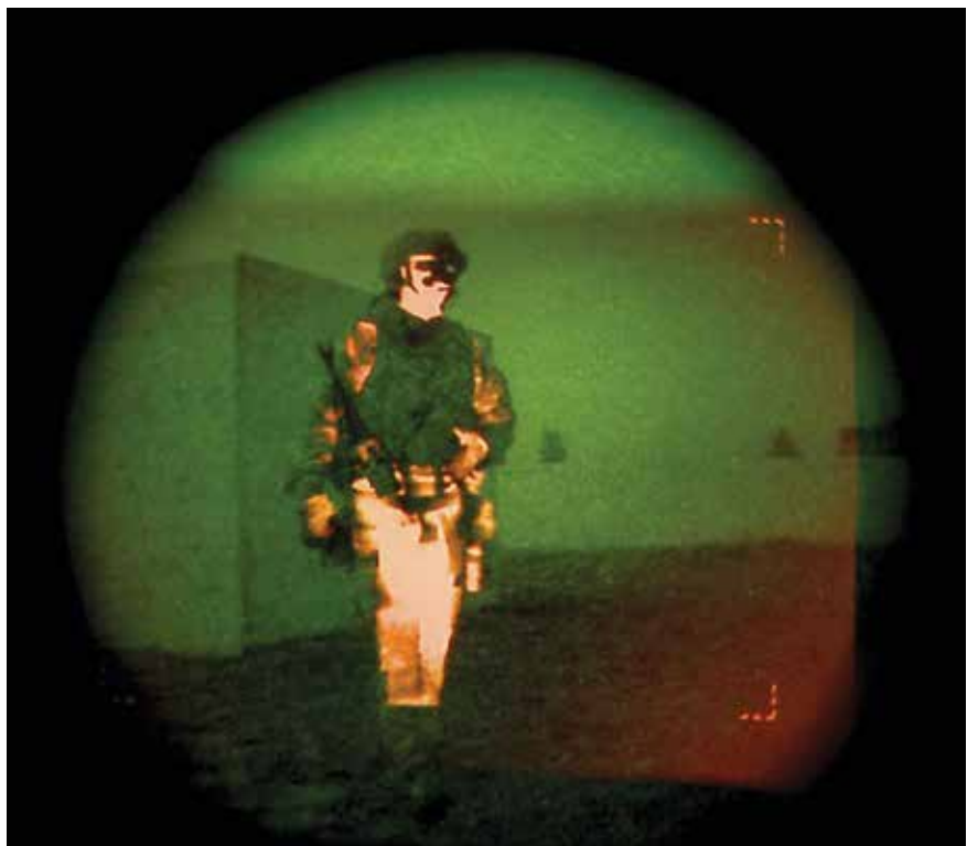
The Enhanced Night Vision Goggle (ENVG) allows several thermal inputs to be fused into a single image.
