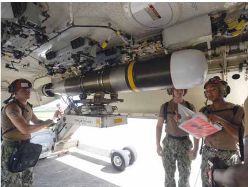
The Mk54 MAKO LWT being loaded on a Boeing P-8A POSEIDON MPRA
