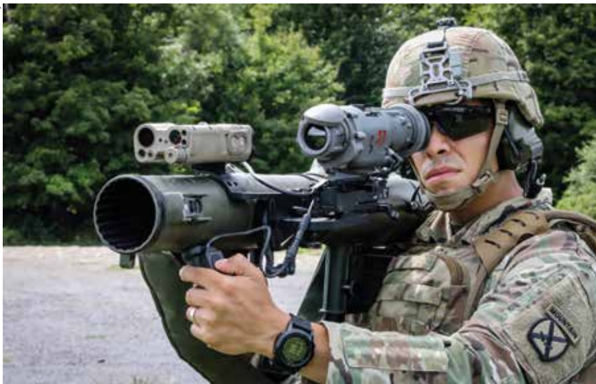
Raytheon's PAS-13, here mounted on a CARL GUSTAV recoilless rifle, is a typical thermal weapon sight.
