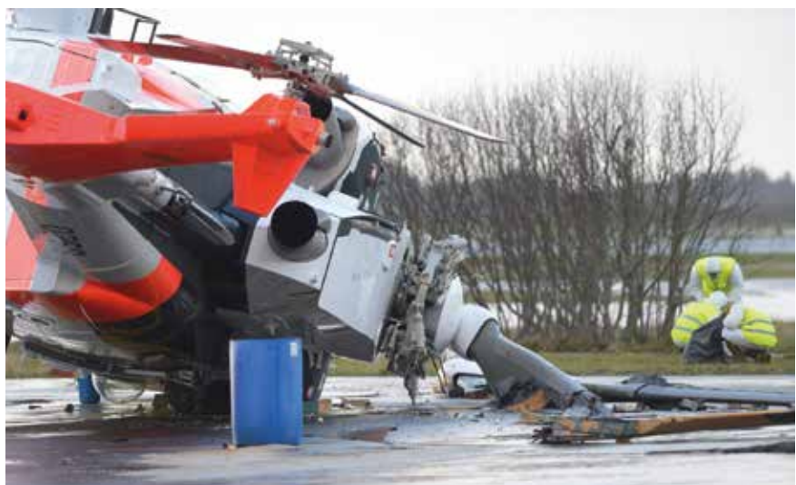
At Sola Air Base, an AW101 helicopter tipped over during maintenance work while the engine and the rotor were running.
