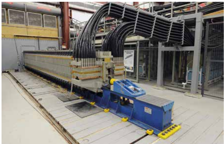
The Office of Naval Research Electromagnetic Railgun located at NSWCDD fired a world-record-setting 33 megajoule shot, breaking the previous record established on 31 January 2008.
