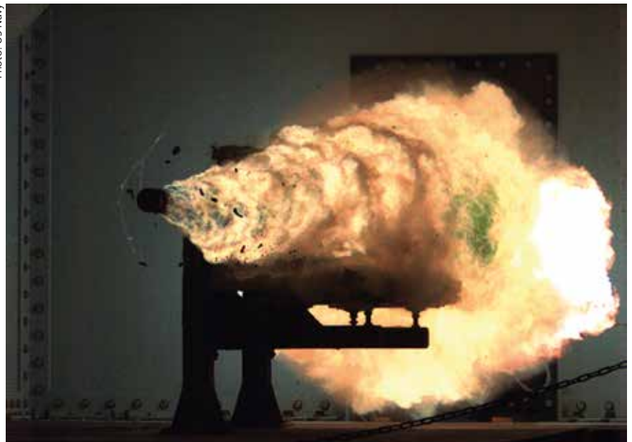
A high-speed video camera captured this image of a test firing of an electromagnetic railgun at the US Naval Surface Warfare Center, Dahlgren, Virginia, in January 2008. The 3.2 kg projectile achieved a muzzle velocity of 2,520 m/sec.
