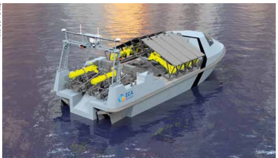
The INSPECTOR family of unmanned surface vehicles (USVs) developed by ECA Group constitute the company's latest solutions for future MCM applications.
