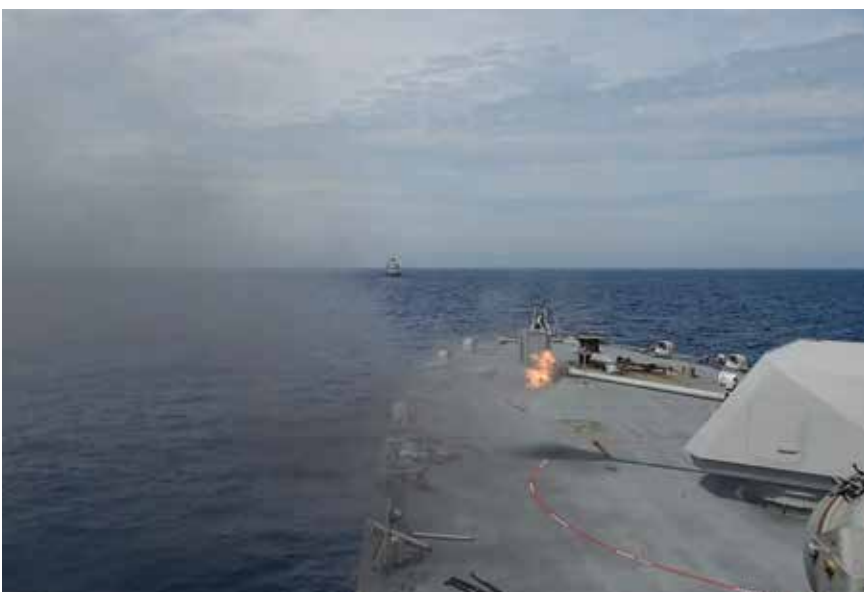
The standard 57mm Mk 110 gun has a 220 round-per-minute rate of fire.
