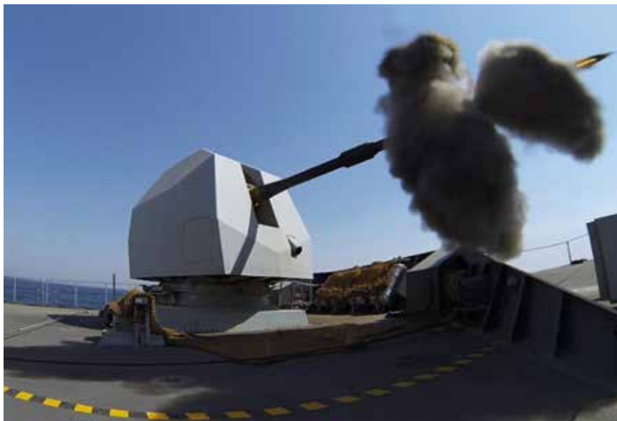
The UK Royal Navy Type 45 destroyer DEFENDER fires its 4.5 inch Mk 8 Mod 1 gun.
