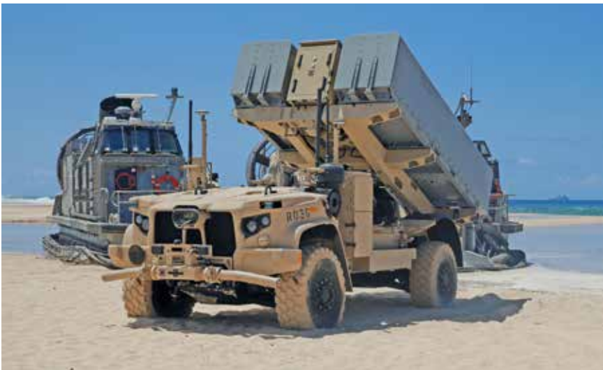
The Navy Marine Expeditionary Ship Interdiction System (NMESIS) launcher provides the USMC with readily deployable anti-ship weapons in support of the EABO concept.
