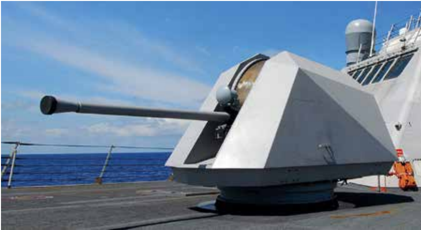
This BAE Systems 57 mm Naval Automatic Gun L/70 is installed on the US Navy's littoral combat ship FREEDOM (LCS-1). Originally developed by Bofors, it has the US designation Mk 110.
