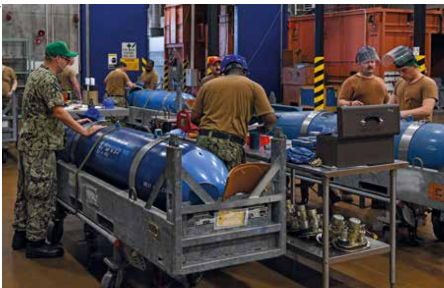
Sailors assigned to Navy Munitions Command East Asia Division Unit Misawa assemble an inert Mk 65 QUICKSTRIKE training mine as part of routine training. A belligerent Russia and the emergence of China as a pacing threat in the Asia-Pacific region are leading the US Navy to think afresh about offensive mining.
