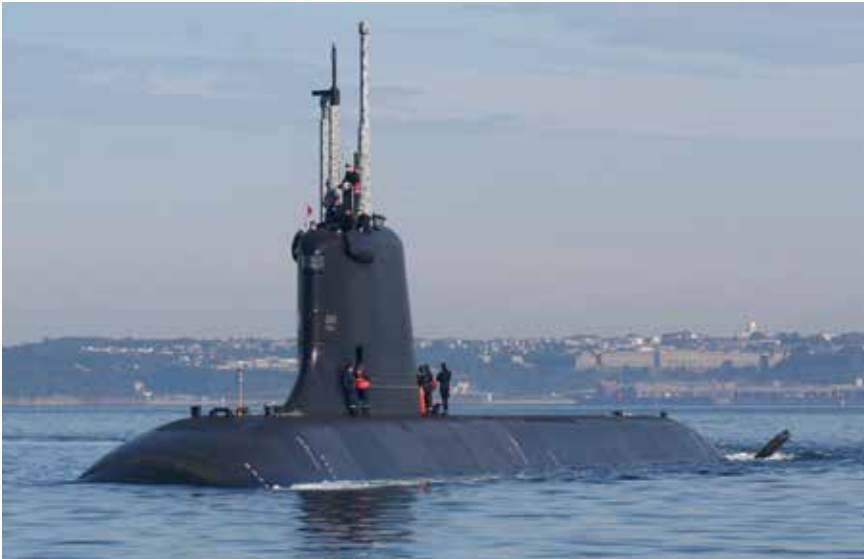
The first of the French Navy's new SUFFREN class nuclear-powered attack submarines pictured off Brest in the course of trials.
