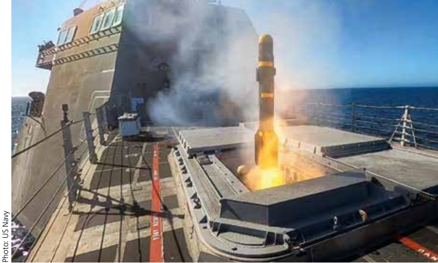
The LCS' ASuW module includes 24 HELLFIRE missiles which can be deployed against swarming boats including fast attack craft. In May 2022, MONTGOMERY became the first LCS to test fire the AGM-114L in the land attack mode, simulating fire support for amphibious forces.
