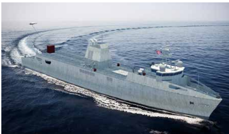
Artist concept of a Large USV with deck-integrated VLS cells, considerable reconfigurable deck space, and a tethered UAV for enhanced situational awareness.
