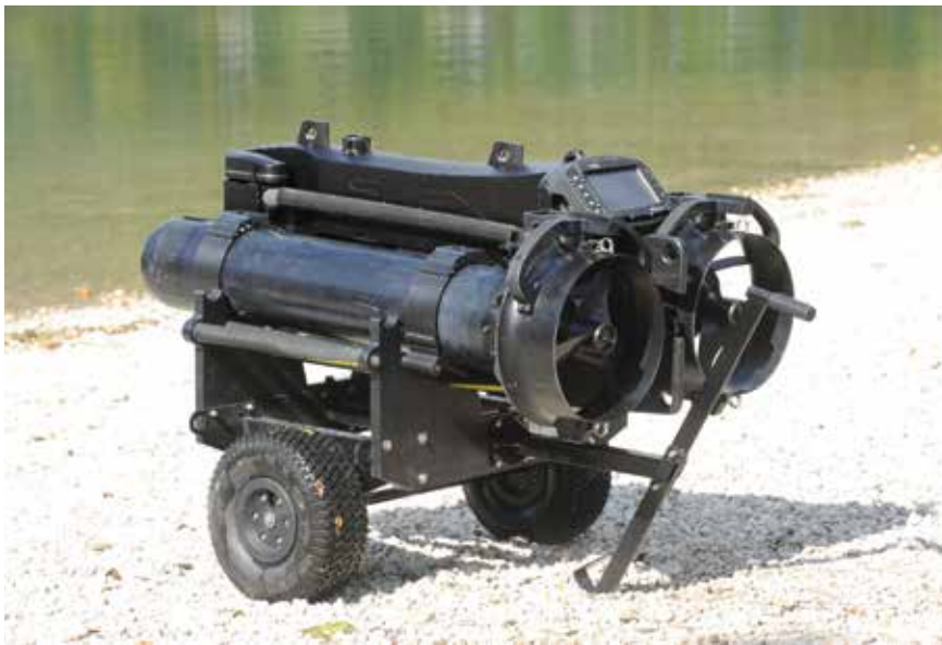
The SUEX Scooter can pull up to four divers or heavy equipment. The DPD transport frame is only for easier transport into the water and is left behind on the beach.
