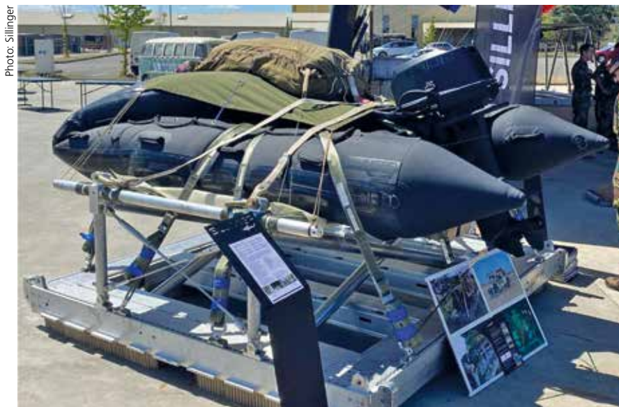
Small Sillinger boat on the Maritime Craft Aerial Delivery System (MCADS) ATAX.
