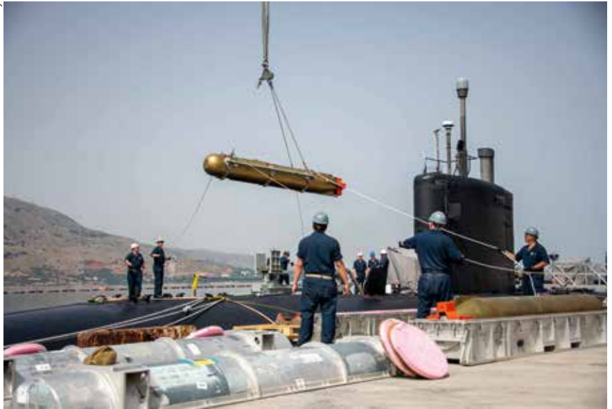
Sailors aboard the LOS ANGELES class submarine MONTPELIER (SSN-765) embark a Mk 77 Submarine Launched Mobile Mine (SLMM) at Souda Bay, Crete in June 2021. The SLMM is launched from submarines in areas inaccessible for other mine deployment techniques.
