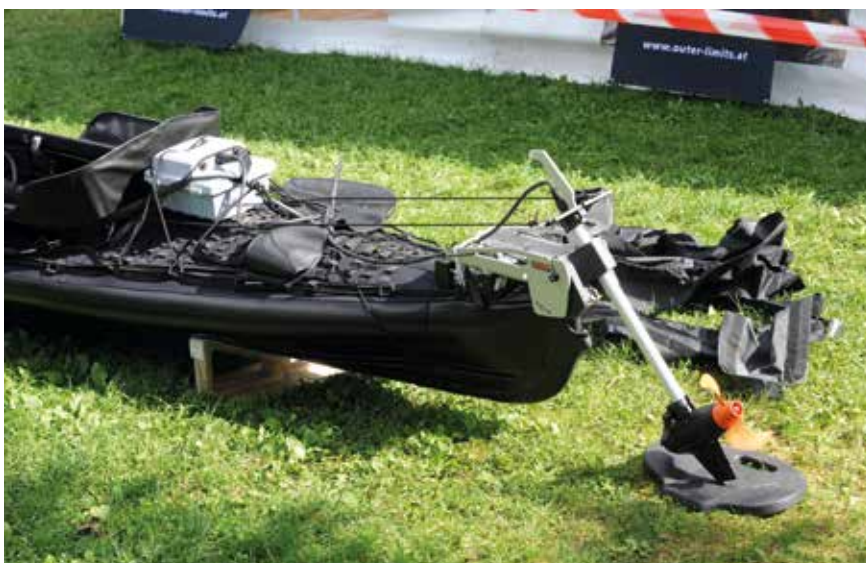
Military kayak by Wayland from Poland with a prototype of an all-electric and silent auxiliary propulsion system.
