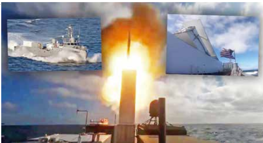
Test firing an SM-6 air-and-missile defence missile from the LUSV prototype RANGER in 2021.
